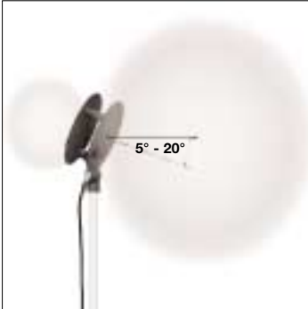
Fig. 4: Hypercardioid polar pattern.
