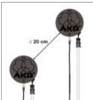
Fig. 8: Minimum distance between two antennas.
